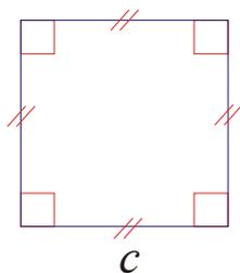
$$\begin{aligned}\mathcal{P} &= c + c + c + c \\ &= 4 \times c\end{aligned}\quad \mathcal{A} = c \times c = c^2$$
